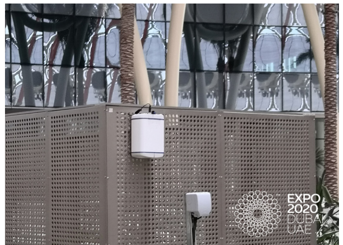
Figure 4: Mains powered Zephyr® monitor deployed outside at Expo 2020 Dubai.
