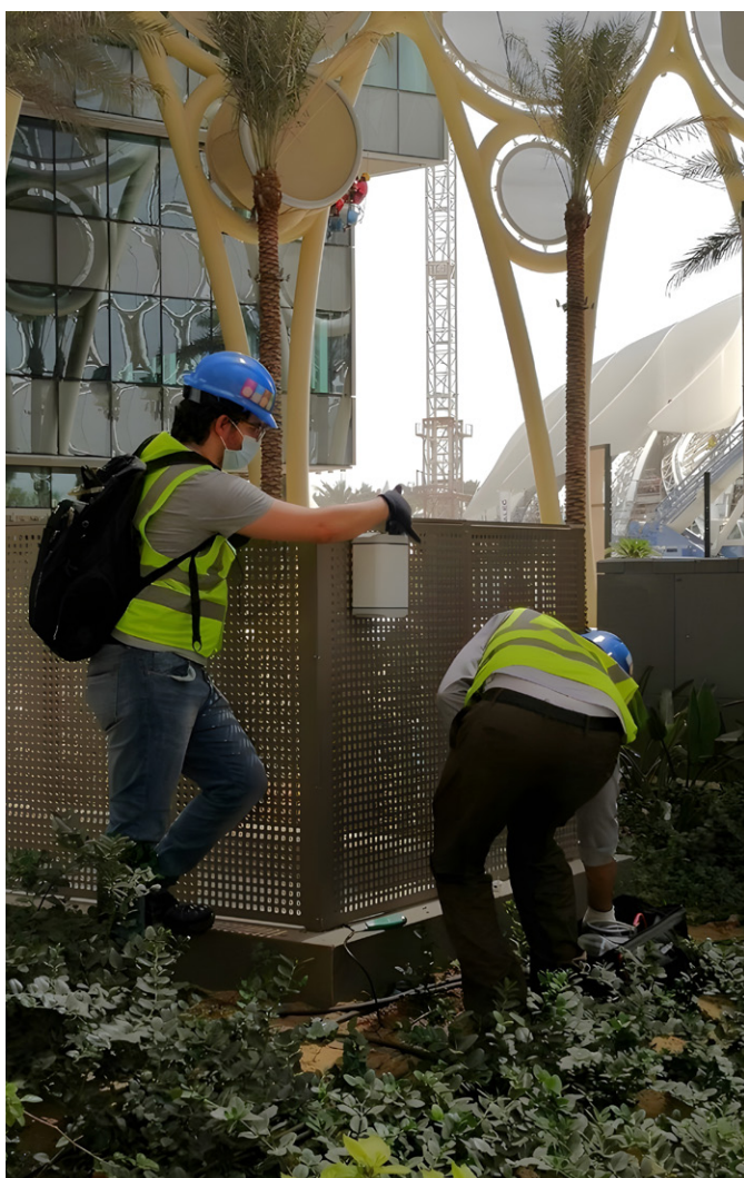
Figure 5: Deployment of a Zephyr® air quality monitor at Expo 2020 in Dubai.
