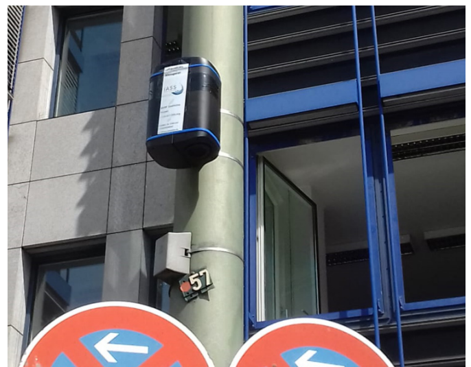
Figure 1: Zephyr® monitor mounted to a lighting column.
