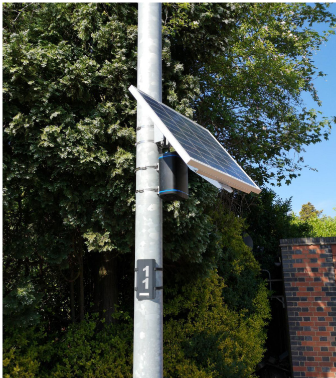
Figure 2: Zephyr® air quality sensor deployed in Leicester to a lighting column powered by solar panel.
